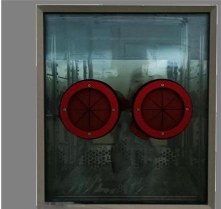
A photograph of a glass door with two red circular observation holes. The holes are set into a dark frame, and the glass behind them shows a blurred interior.                                     | <p>从内门观测、操作试验槽内部的试料。</p> <p>操作孔：一对、两对</p> <p>*可能会对标准性能有影响，详情请咨询销售公司。</p> <p>*试验槽观测视窗凹进约 45mm.</p>                                |
