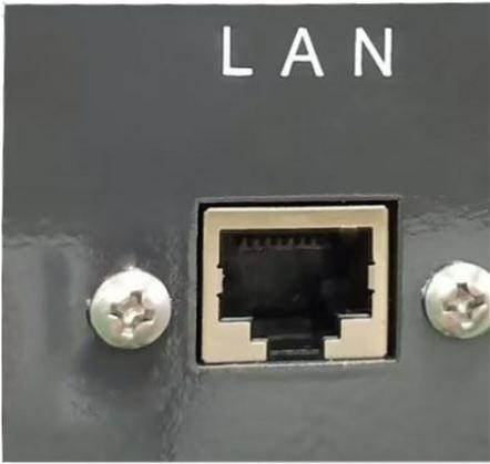
A close-up photograph of a grey metal panel featuring a central RJ45 LAN port. Above the port, the letters 'LAN' are printed in white. Two silver screws are positioned on either side of the port. | <p>电脑与设备连接，用通讯协议设置（定值，程序）运转的变更，监控，自动化等。可选项：<br/>Web(lan)/RS-485/RS-232C</p>                                                      |
